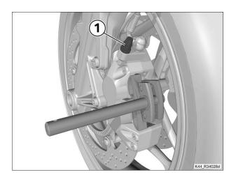
not possible to tell whether the brake fluid extracted from the system is free of bubbles.
