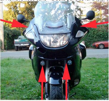
you will also need to pry it up and out as it pressed into the fairing. I found the easiest thing to do was to wedge my finger between the fairing and the windscreen and pry up (see below)
