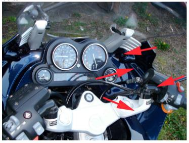
2. Remove nose cone – 2 bolts per side for a total of 4 bolts
