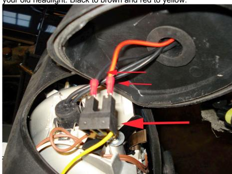
9. Close headlight back up and secure wire on back panel
